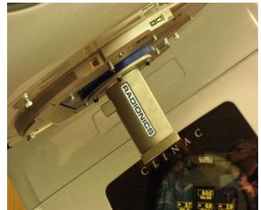
*Cone attachment onto Linac machine at Dunedin Hospital*
